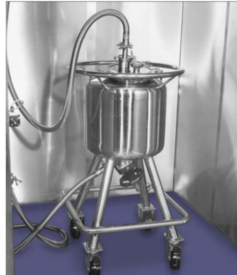
Vessel in Enclosure for SIP
