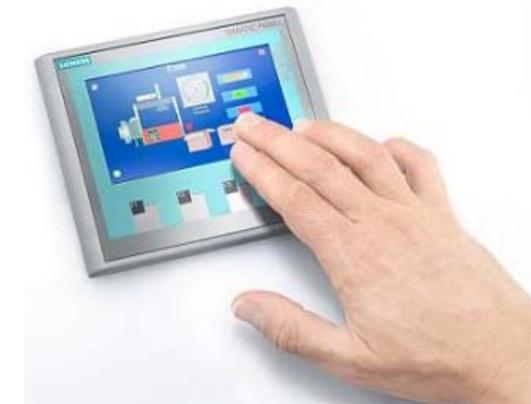
**CIPSuite#2000™** - Automatic control system with 20 fully configurable recipes, I/O faceplates, mimic diagrams, profibus, ethernet and hard wired interfaces, optional printer & datalogger, repeatable automatic cycles, User control with passwords, In built troubleshooting and diagnostic ability.
