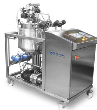
Designed to comply with ASME BPE (Bioprocessing Equipment) – the international standard for the design and construction of equipment intended for use in the manufacturing of biopharmaceuticals – they include compliance with the '2D deadleg' rule, an area of entrapment in a vessel or piping run that could lead to contamination of the product. The system also offers full drainability, full traceability and is completely validatable
